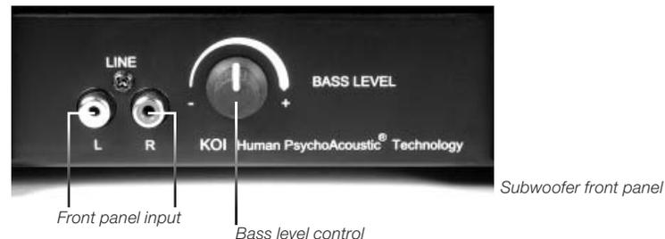
There are three sets of stereo inputs on the Tiger. The **Line** input on the front panel and the **Aux** input on the rear panel of the subwoofer are recommended for use with most consumer audio equipment. The **Audio** input on the rear panel is better suited for pro audio equipment with standard 0dBu (.775V) line-level output.
