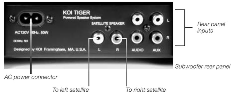
If necessary, you can purchase longer speaker cables pre-wired with RCA-type phono connectors at most electronics supply stores, such as Radio Shack. Do **not** use shielded cables for this purpose as they may adversely affect audio performance.
